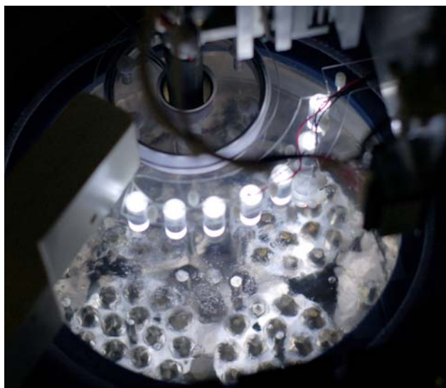
Figure 1. The illuminated cryopuck storage Dewar with its transparent monolithic lid.
