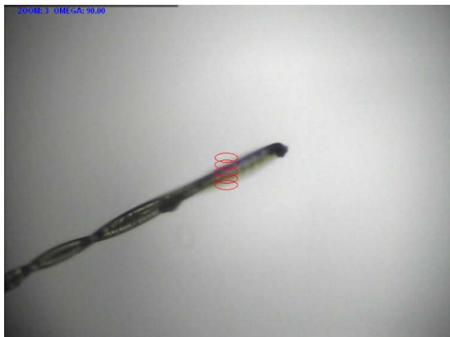
Fig. 4 Visual of the Occluded View Alignment with the edge of loop aligned with the plane of view. Note the inability to visually detect the location of the thin crystal. Red ellipses show areas of impending X-ray diffraction.
