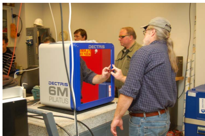
Fig. 2 Malcolm Capel passes a weakly radioactive Fe-source over the front of the PILATUS-6MF to test sensitivity during commissioning.
