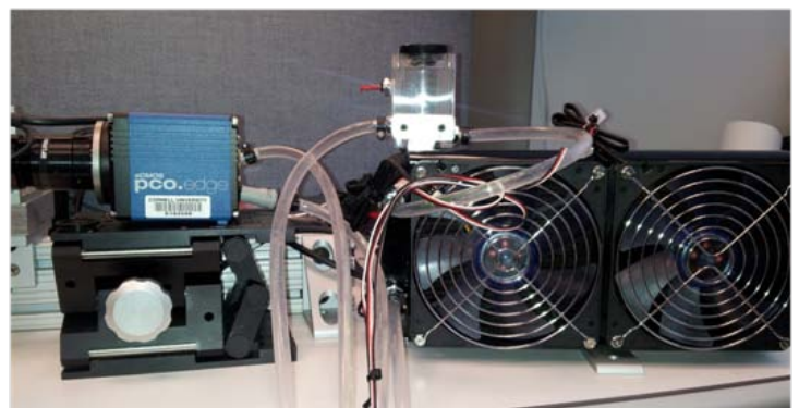
Fig. 5 A) sCMOS Camera in December 2013. B) sCMOS camera refitted with water cooling of its Peltier.
