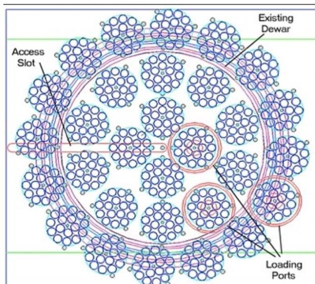
**Fig. 1** CAD drawing of sample locations for the proposed 30-puck high capacity automounter.
