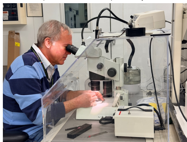
Figure 5 Harvesting crystals in a repurposed fume hood. The 'portable' fume hood was salvaged from cleanup efforts around the APS. It is still very heavy and not easy to move around.
