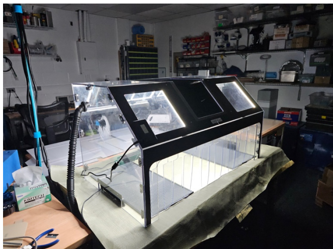
Figure 6 Initial build of a portable humidity chamber at MiTeGen.
