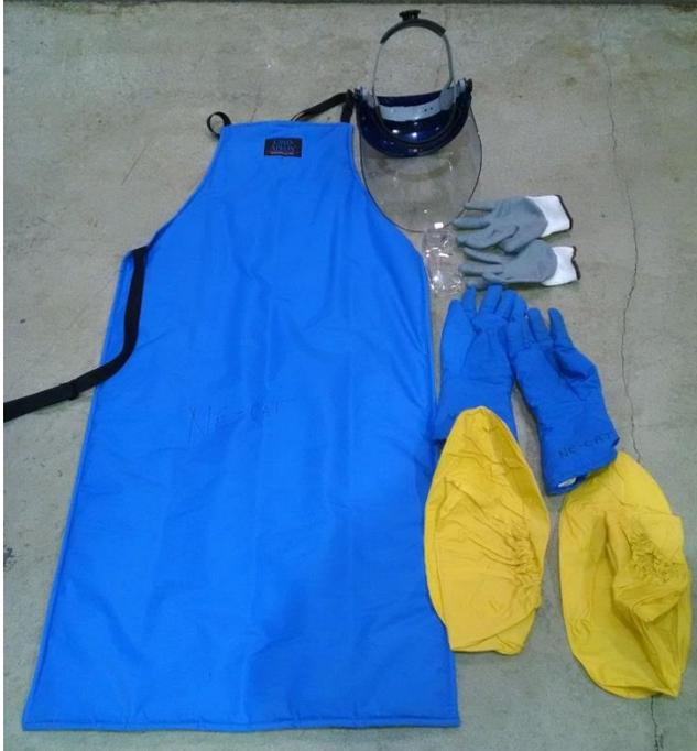
2. Wear the **PERSONAL PROTECTIVE EQUIPMENT (PPE)**. PPE (safety glass, face shield, shoe covers, cryogenic gloves and apron) must be worn while operating LN2 filling station.
