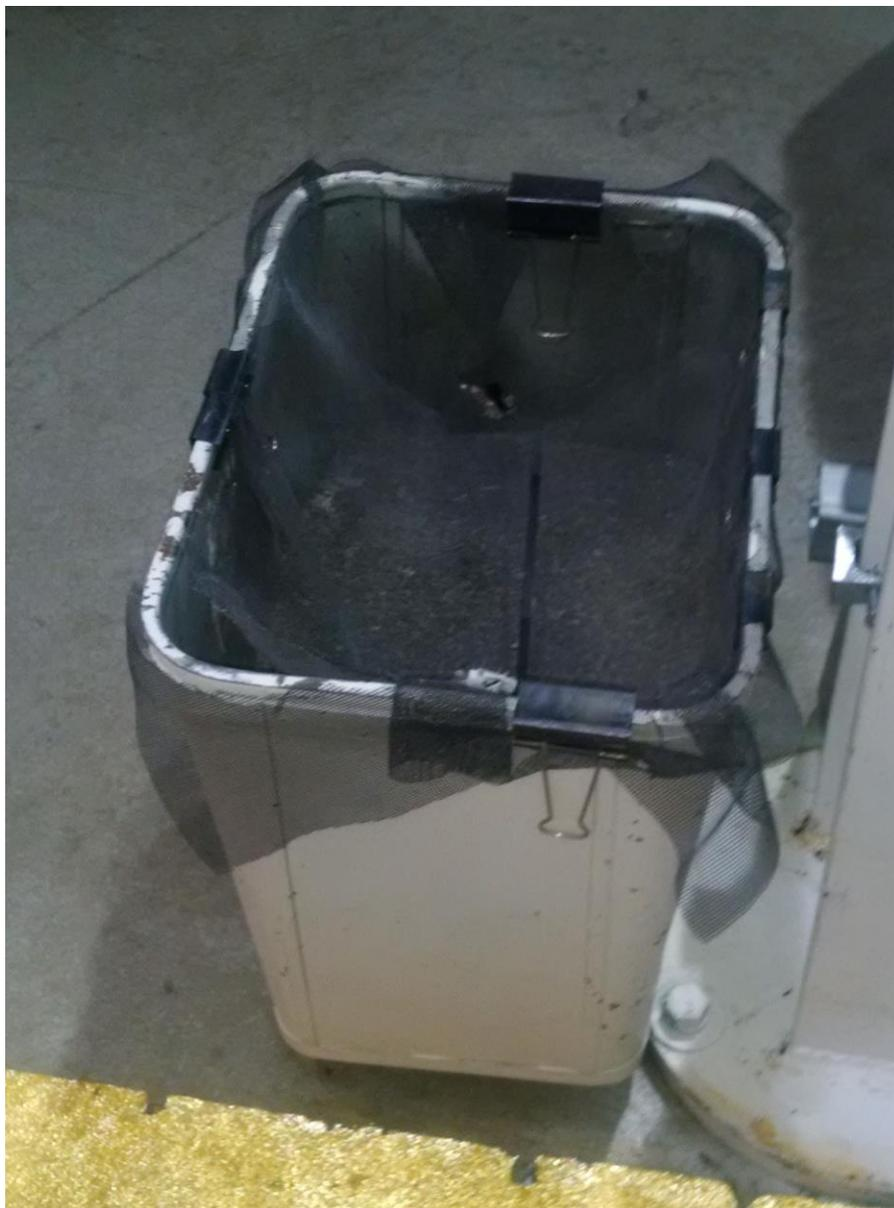
6. Dispose the extra LN<sub>2</sub> in the waste container carefully.
