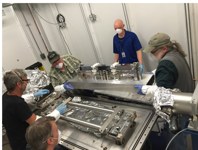
Fig. 4 Placement of the 24-ID-C VFM on the transition assembly. Shipping restraints hold the mirror in place over the support structure and cams. Clockwise from top left: Ed Lynch, Jon Schuermann, Malcolm Capel, Frank Murphy, Ian Campton.
